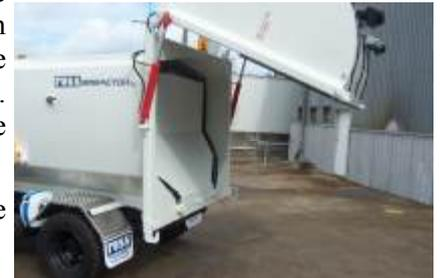
Strong lightweight aluminium mudguards fitted with white mudflaps finish the unit off.
